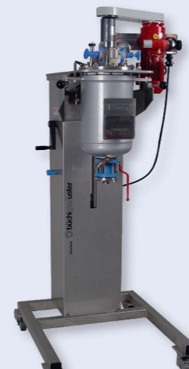
kiloclave inert, bmd 250 «i» ATEX glass lined steel reactor: 10 Liter, 6 bar, 180°C Stahl Emaille Reaktor: 10 Liter, 6 bar, 180°C
